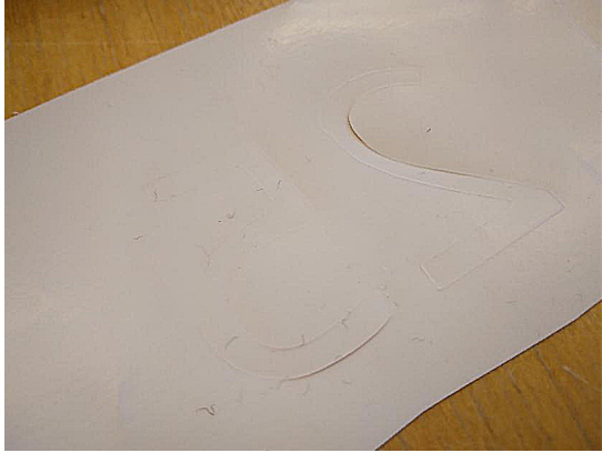
Figure 8: Vinyl with a pattern cut out
