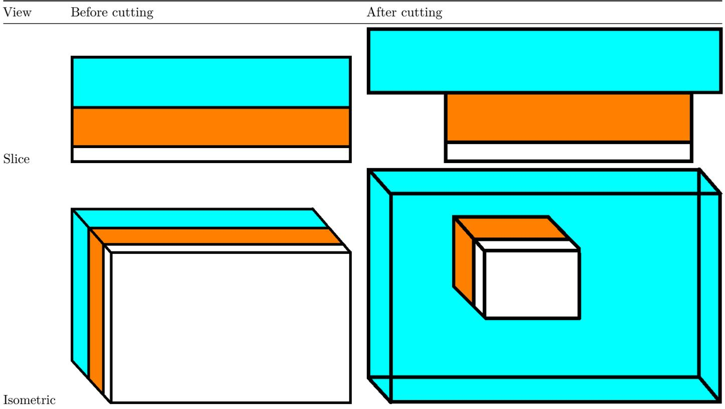
Structure of the foil and what will be cut away. Light-blue: thick, transparent layer, do not cut, can be separated from orange layer by hand. Orange: the color of the print. White: the glue connecting the print to the T-shirt
