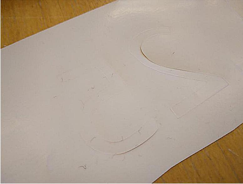
Figure 8: Vinyl with a pattern cut out
