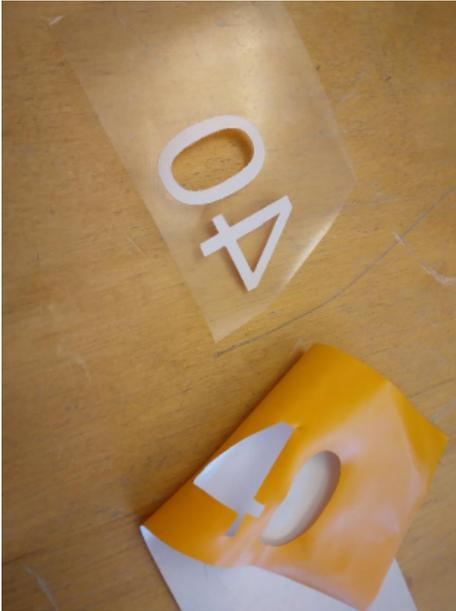
Figure 3: Transfer foil ready for transfer
