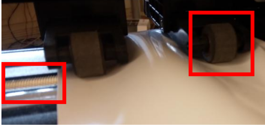
Figure 13: The right wheel is not on the roller
