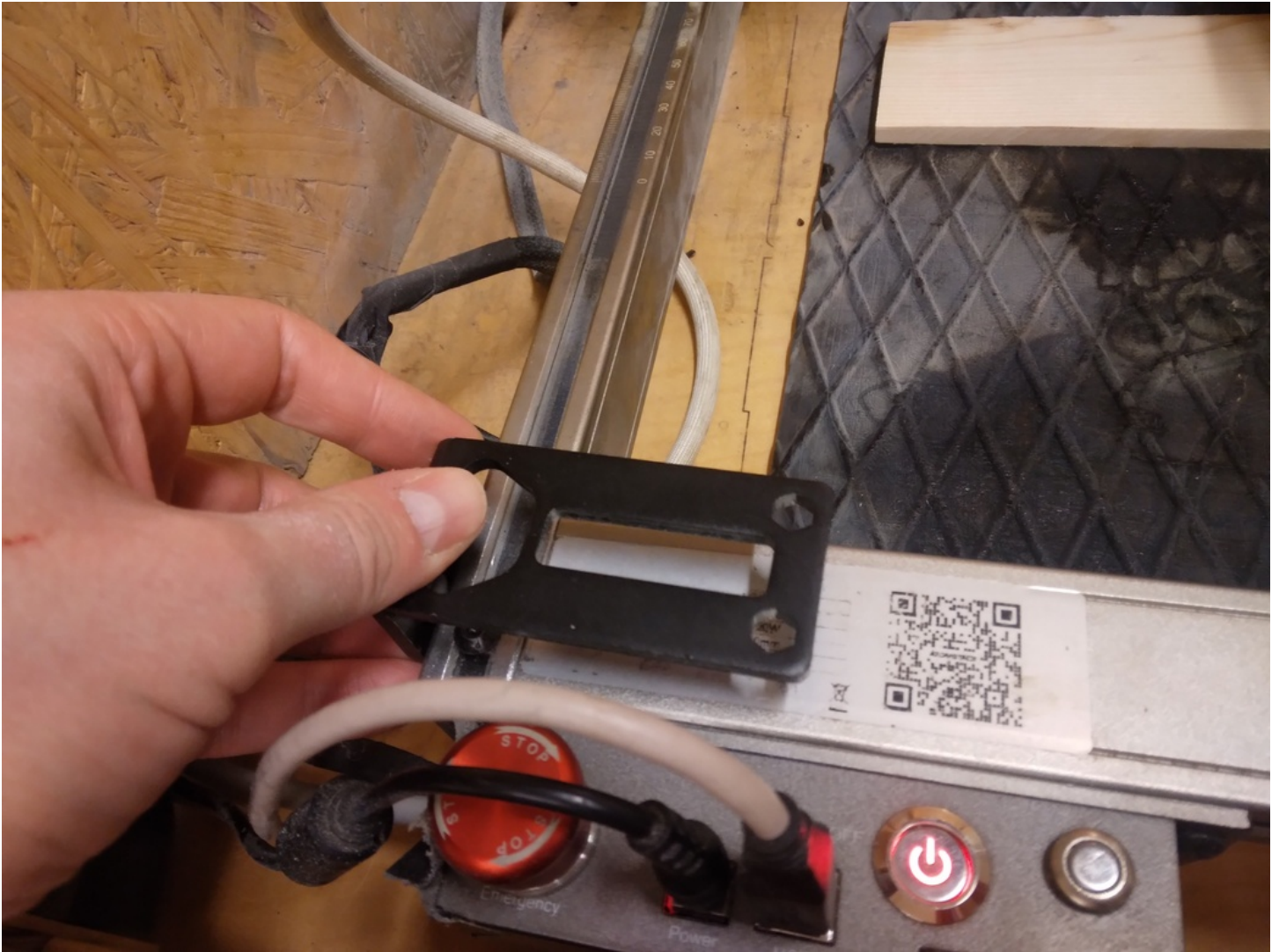
Figure 20: Take the spacer from its proper place.
